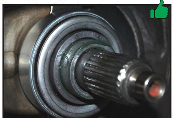
Example of PERFECT AMOUNT OF GREASE on the input shaft. As you can see, it is barely visible to the naked eye and acts as more of a lubricant.
